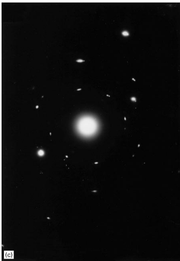
Figure 6 Transmission electron micrographs of low alloy CrMo steel austenized at 1123 K and tempered at 973 K. (a) Bright-field image, (b) dark-field image of cementite, (c) selected area diffraction pattern in (a) with the cementite orientation spot, (d) analysis of the SAD pattern in (c).
