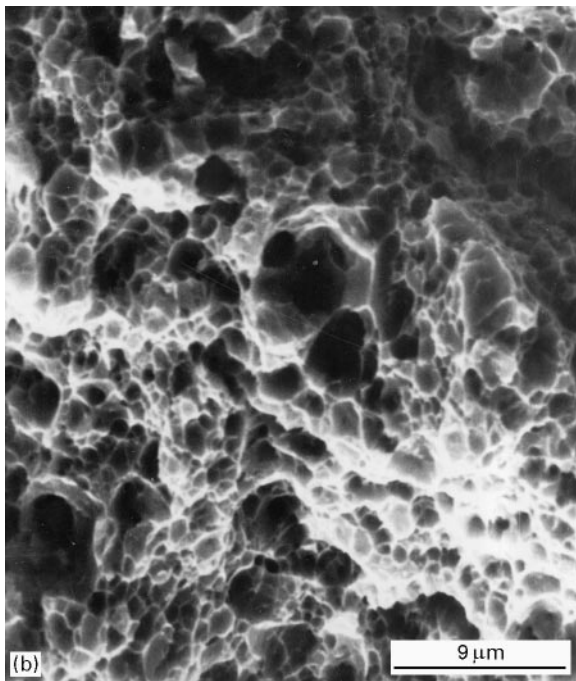
Figure 10 Scanning electron microscopy fractographs of low alloy Cr (a) and CrMo (b) steel tempered at 973 K.
